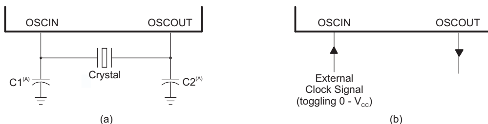
Figure 7-2. Crystal/Clock Connection
